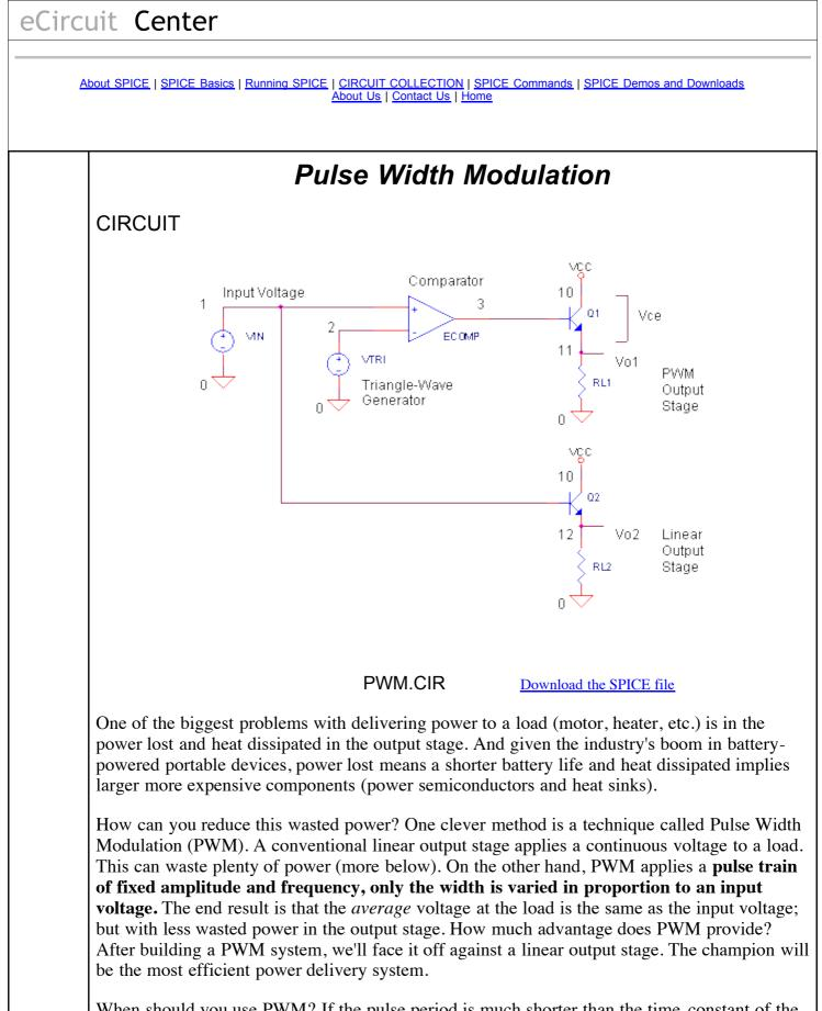
When should you use PWM? If the pulse period is much shorter than the time-constant of the load, then PWM has a potential application. The time-constants are defined, for example, by the thermal mass of a resistive heater or the mechanical inertia of a motor. And it's the long
