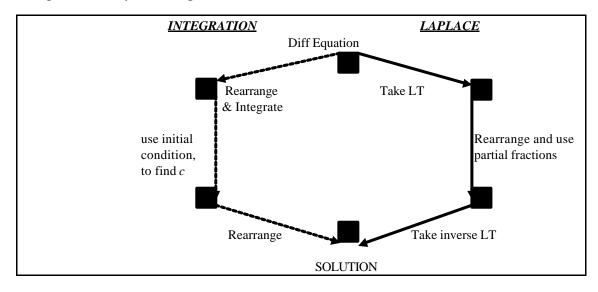
This doesn't look too big a deal, since the LT method used the unexplained variable, *s*, and needed the use of partial fractions. However, in reviewing the two solutions above you can see that in the LT method there is no need to use integration, the constant of integration is automatically found and there was no messy rearrangement of exponential equations required.
