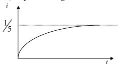
Note that the current settles down to a *steady-state* value of one-fifth of an amp and has a *time constant*, *t*, of one-fifth of a second - the *transient* (that part of the solution relating to the exponential decay) dies away in about one second.
