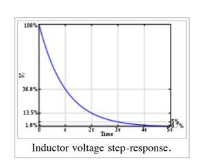
in the circuit is changing — as the circuit reaches its steady-state, there is no further current change and ultimately no inductor voltage.
