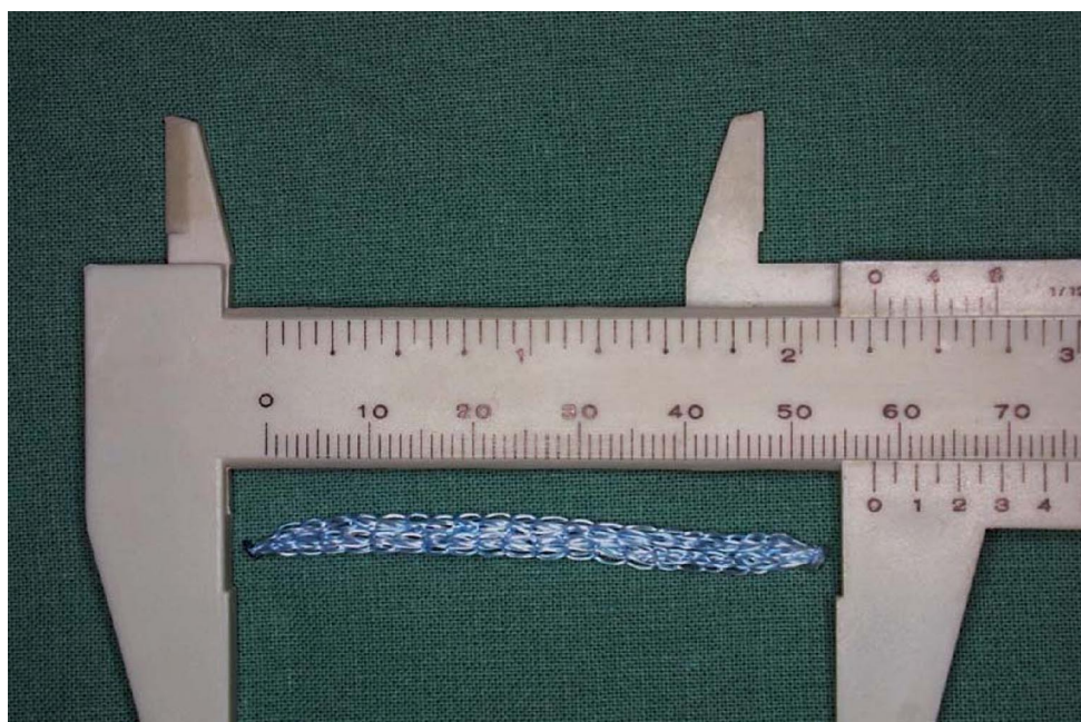
Figure 1. Knitted structure of PLLA and PLGA. This figure is published in colour on http://www.ingenta.com
