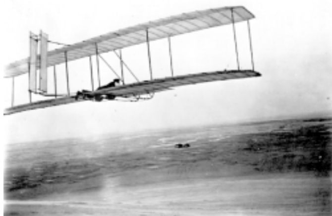
Figure 37. Testing the two-surface rudder on the 1902 glider in October 1903.
