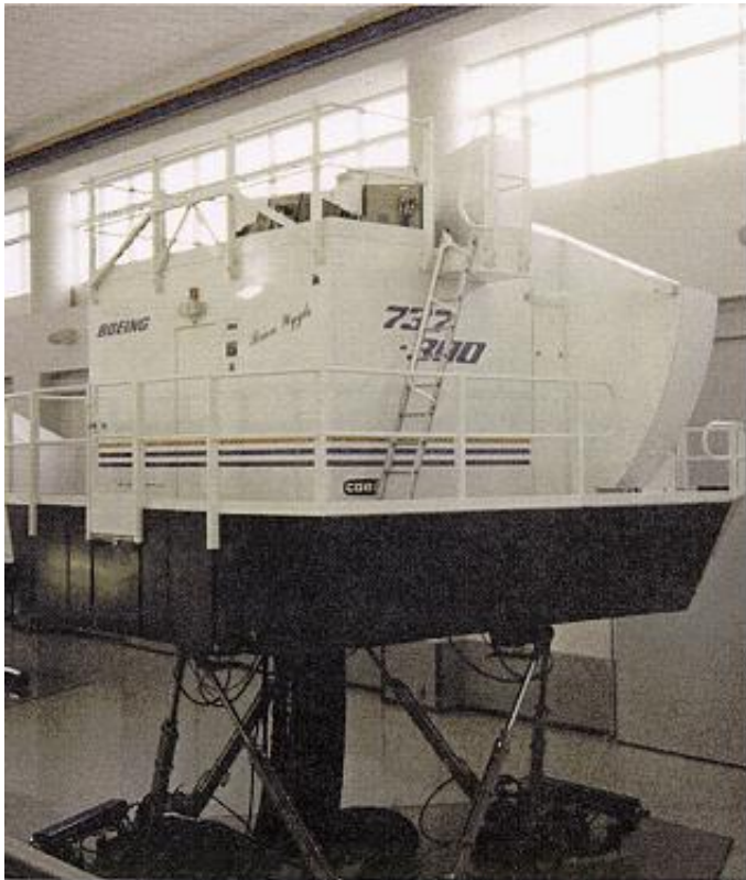
Figure 2.2.5.1 – A 737-300 Simulator with 6 DoF
