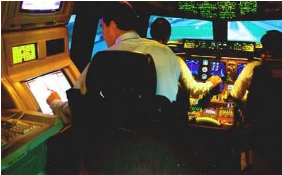
Figure 2.2.2.1 – A typical IOS layout within a simulator. Note the touch screen implementation
