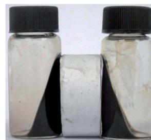
**Fig. 5** Photographs of the ferrofluidic behavior of 12 nm OA-stabilized NPs in hexane (left) and 12 nm PAIONs in water (right).
