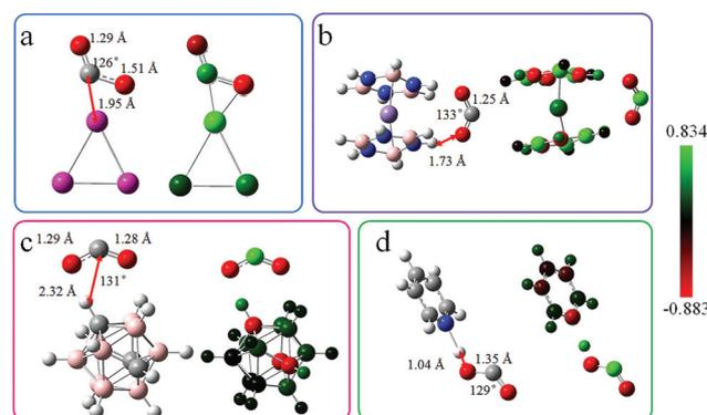
Fig. 3 (a) to (d) Optimized geometries (left panel) and NBO charge distribution (right panel) of four different kinds of neutral superalkalis interacting with the  $CO_2$  molecule.
