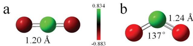
Fig. 2 Optimized geometries with bond angles and CO bond distances, and the NBO charge distribution in (a) neutral  $CO_2$  and (b)  $CO_2^-$  anion.
