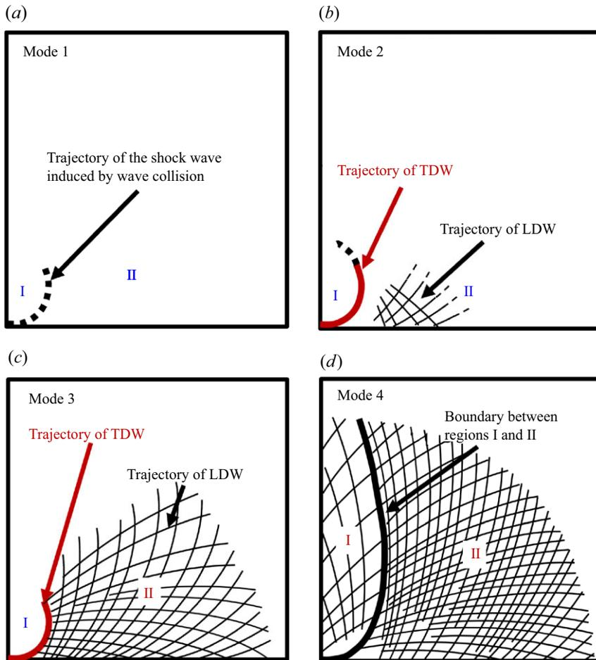
Figure 7. Schematics of typical detonation initiation modes. (a) Mode 1, (b) mode 2, (c) mode 3 and (d) mode 4. Region I is dominated by hot spot autoignition, and region II is determined by wave collisions. Black dash lines in mode 2 represent the trajectories of the decoupled TDW and LDW. LDW: longitudinal detonation wave; TDW: transverse detonation wave.
