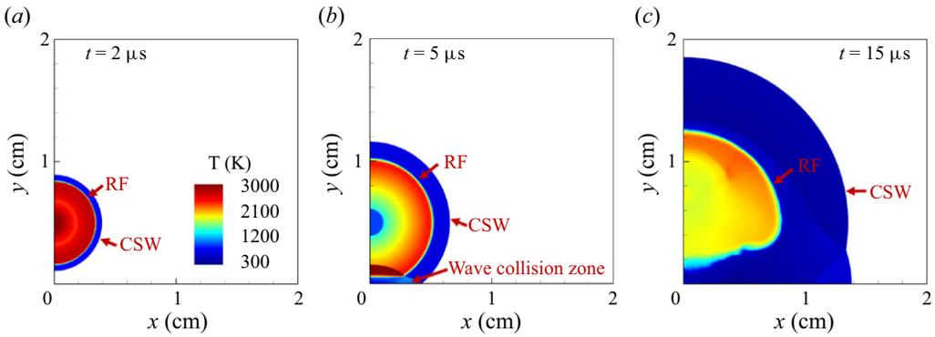
Figure 4. The temporal evolution of temperature contour during the detonation initiation process for  $P_h = 15$  atm and  $L = 10$  mm. Panels show (a)  $t = 2 \mu\text{s}$ , (b)  $t = 5 \mu\text{s}$  and (c)  $t = 15 \mu\text{s}$ . CSW: cylindrical shock wave; RF: reaction front.
