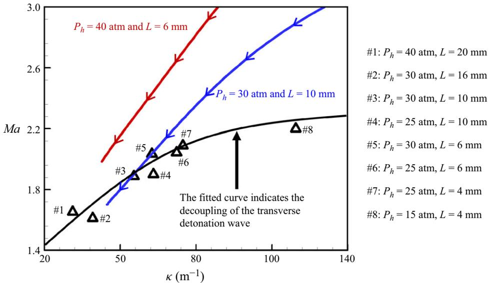
Figure 16. Mach number of the CSW changes with the curvature of triple-point path during the triple-point moving process (the blue line is for  $L = 10$  mm and  $P_h = 30$  atm, and the red line is for  $L = 6$  mm and  $P_h = 40$  atm). The symbol ( $\rho$ ) represents the state when the TDWs decouple for the different cases. The black fitted curve indicates the empirical boundary for TDW decoupling.
