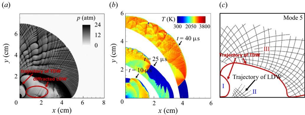
Figure 8. Detonation initiation process for  $P_h = 30$  atm and  $L = 4$  mm. (a) Numerical soot foil, (b) temporal temperature contours near the wave front and (c) schematic of detonation initiation mode. Region I is dominated by hot spot autoignition, region II is determined by CSW collisions and region III is dominated by TDW collision.
