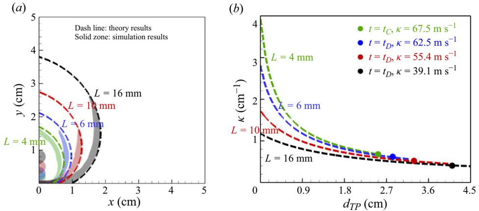
Figure 13. (a) Simulated TDW and theoretical triple-point trajectories; (b) change of the curvature of the triple-point trajectory,  $\kappa$ , with its moving distance,  $d_{TP}$ , during the detonation initiation processes for  $P_h = 30$  atm and  $L = 4, 6, 10$  and  $16$  mm.
