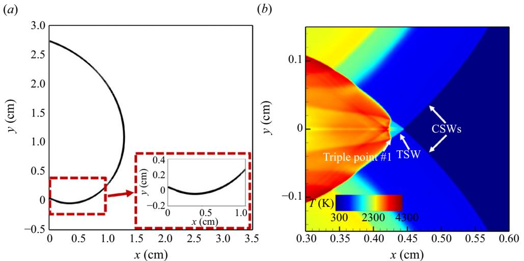
Figure 19. (a) Theoretical triple-point trajectory and (b) simulated temperature contour near the x-axis at  $t = 4 \mu\text{s}$  for the detonation initiation process  $P_h = 30 \text{ atm}$  and  $L = 10 \text{ mm}$ .
