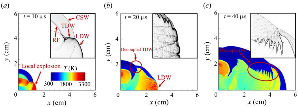
Figure 5. The temporal evolution of temperature contour and wave structure (inset) during the detonation initiation process for  $P_h = 25$  atm and  $L = 10$  mm. Panels show (a)  $t = 10 \mu\text{s}$ , (b)  $t = 20 \mu\text{s}$  and (c)  $t = 40 \mu\text{s}$ . LDW: longitudinal detonation wave; TDW: transverse detonation wave; CSW: cylindrical shock wave; RF: reaction front.
