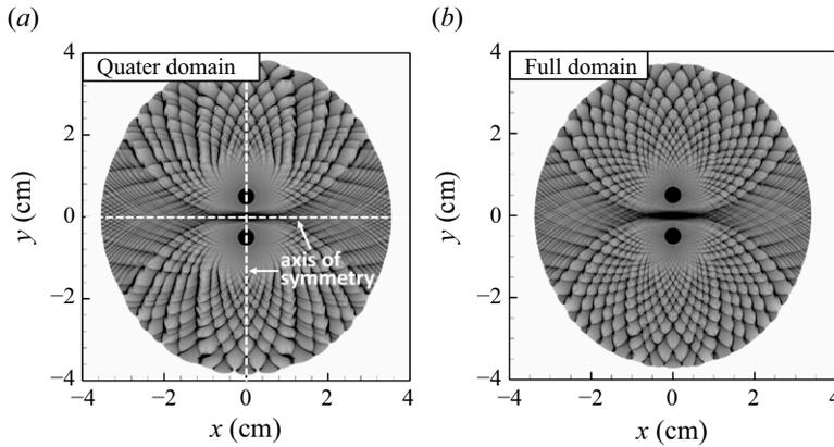
Figure 17. Numerical soot foils depicting the detonation initiation and propagation processes, predicted using (a) the quarter-domain set-up with symmetry boundary conditions and (b) the full-domain set-up. Here,  $P_h = 60$  atm and  $L = 10$  mm.
