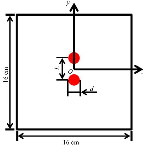
Figure 1. Schematic diagram of the computational domain.
