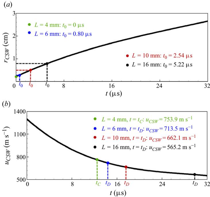
Figure 12. The temporal evolution of the (a) radius and (b) propagation velocity of the expanding cylindrical shock induced by a single hot spot autoignition with  $P_h = 30$  atm and  $T_h = 3000$  K. Here,  $t_0$  is determined by condition  $r_{CSW} = L/2$ ,  $t_C$  is the time when TDW collides on the  $y$ -axis and  $t_D$  is the time when TDW decouples.
