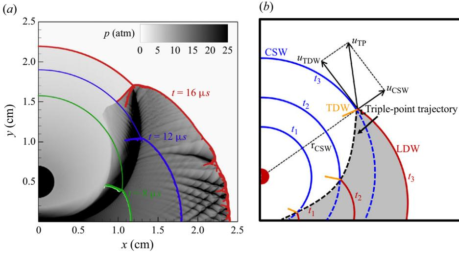
Figure 11. (a) The numerical soot foil at  $t = 16 \mu\text{s}$  and wave fronts at  $t = 8, 12$  and  $16 \mu\text{s}$  for  $P_h = 30 \text{ atm}$  and  $L = 10 \text{ mm}$ ; (b) schematic of temporal wave structures during the detonation initiation process.
