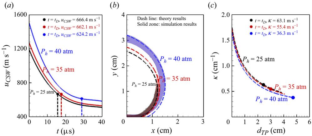
Figure 14. (a) Propagation velocities of the expanding CSWs; (b) simulated TDW and theoretical triple-point trajectories; (c) theoretical curvatures of the triple-point path vary with its moving distance during the detonation initiation processes. Different hot spot pressure of  $P_h = 25, 30$  and  $40$  atm are considered, while  $L$  is fixed to  $10$  mm.
