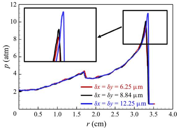
Figure 3. Average pressure distribution along the radius within the fan-shaped region (see [figure 2\(a\)](#)) predicted using different grid sizes.
