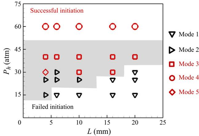
Figure 15. Detonation initiation modes in  $P_h$ - $L$  diagram for hot spot pressure ( $P_h$ ) ranging from 15 to 60 atm and hot spot distance ( $L$ ) ranging from 4 to 20 mm. Critical cases corresponding to modes 2, 3 and 5 are within the grey zone.
