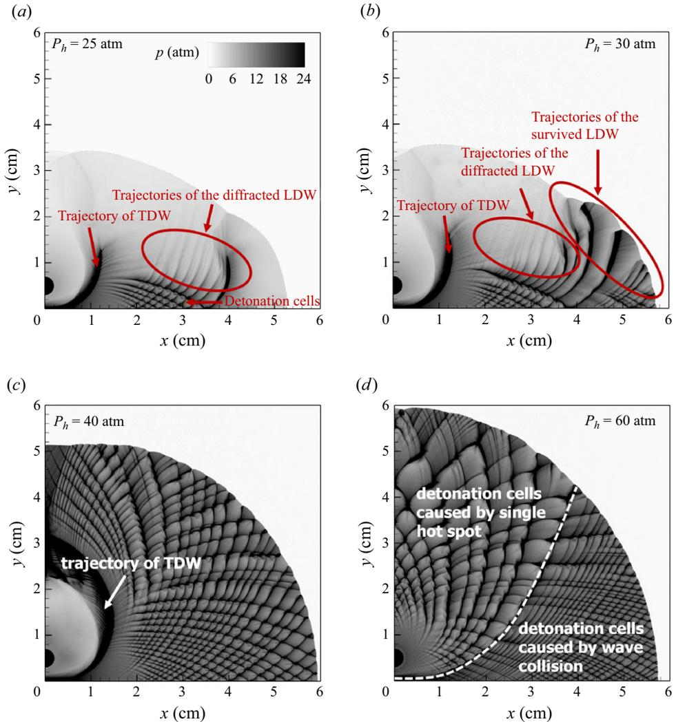
Figure 6. Numerical soot foils for the detonation initiation at different hot spot pressures: (a)  $P_h = 25$  atm, (b)  $P_h = 30$  atm, (c)  $P_h = 40$  atm and (d)  $P_h = 60$  atm. The hot spot distance is fixed to be  $L = 10$  mm. LDW: longitudinal detonation wave; TDW: transverse detonation wave.
