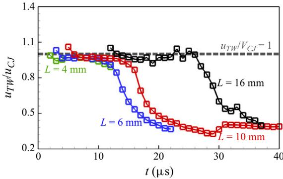
Figure 18. Propagation speeds of the transverse wave under different distances ( $L = 4, 6, 10$  and  $16$  mm) between the dual hot spots. Hot spot pressure is fixed at  $30$  atm.
