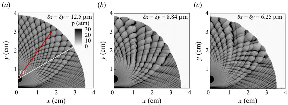
Figure 2. Numerical soot foil for detonation initiation and propagation process with  $P_h = 60$  atm and  $L = 10$  mm. The minimum grid sizes are: (a)  $\delta x = \delta y = 12.5 \mu\text{m}$ ; (b)  $\delta x = \delta y = 8.84 \mu\text{m}$ ; (c)  $\delta x = \delta y = 6.25 \mu\text{m}$ .
