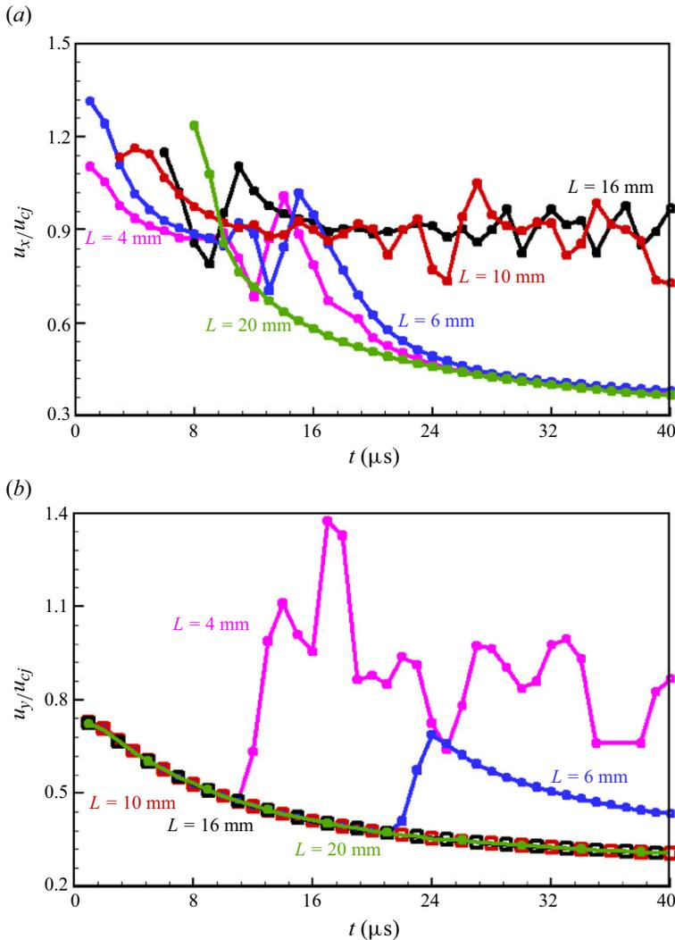
Figure 10. Normalised leading shock wave speeds along (a) the  $x$ -axis and (b) the  $y$ -axis during the detonation initiation processes for  $L = 4, 6, 10, 16$  and  $20$  mm and  $P_h = 30$  atm.
