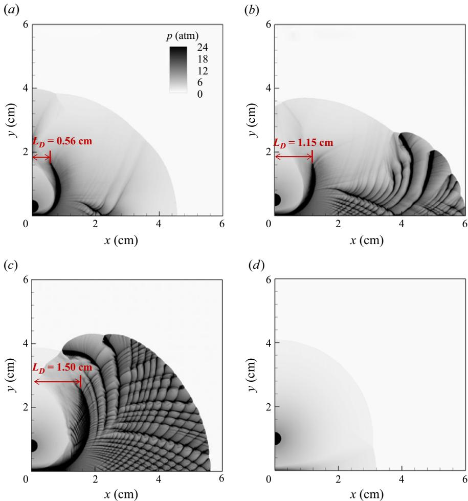
Figure 9. Numerical soot foils for detonation initiation at different hot spot distances: (a)  $L = 6$  mm, (b)  $L = 10$  mm, (c)  $L = 16$  mm and (d)  $L = 20$  mm. The hot spot pressure is fixed to be  $P_h = 30$  atm.  $L_D$  is defined as the distance from the transverse wave decouple location to the  $y$ -axis.
